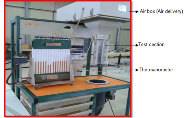
(b) Photo graph of used test rig
